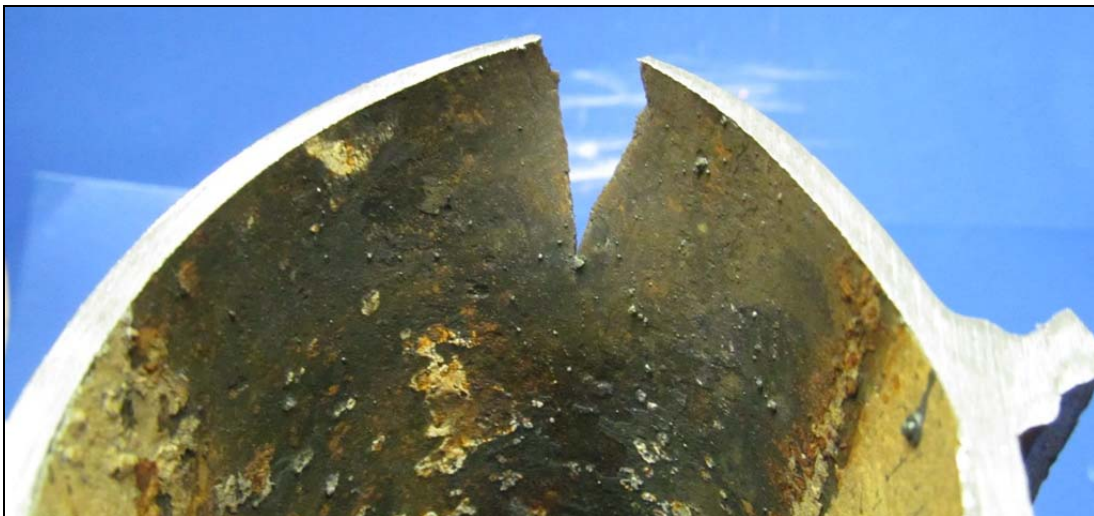
Figure 3: Photograph displaying the failure of Tube #69. The failure exhibited a mild fish-mouth morphology. Further analysis would find that the failed region had been overheated at the time of failure.
